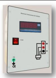
Digital Instrument that, coupled to an optical speed transducer, Allows measuring the rotating speed of electrical machines
